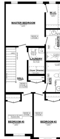
ASHTON 'C' UNIT #3 2ND FLOOR PLAN 910 SQ. FT. 8' CEILINGS ON 2ND FLOOR
