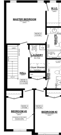
ASHTON 'A' UNIT #1 END 2ND FLOOR PLAN 910 SQ. FT. 8' CEILINGS ON 2ND FLOOR
