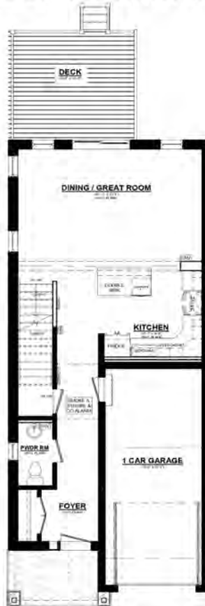
Ashton B UNIT #1 MAINFLOOR PLAN 690 SQ. FT. 8' CEILINGS ON MAINFLOOR CEILINGS ON MAINFLOOR
