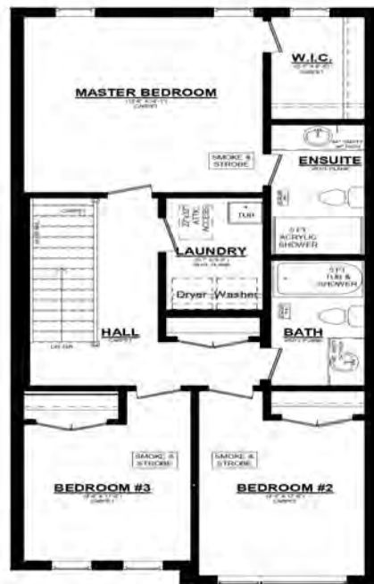
Ashton B UNIT #1 2ND FLOOR PLAN PLAN 910 SQ. FT. 8' CEILINGS ON 2ND FLOOR' CEILINGS ON 2ND FLOOR PLAN
